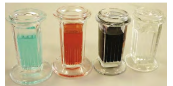
3) Stain Rapid staining: immerse in fixative and then in each stain 5 x 1 sec. each
